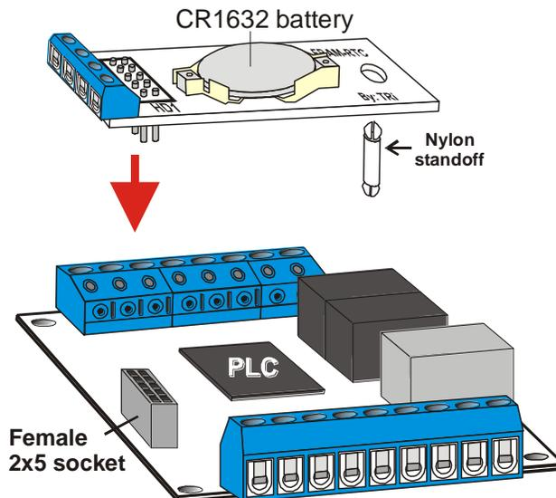
To install the I2C-FRTC module, first **ensure that you have turned OFF** power to the PLC.
