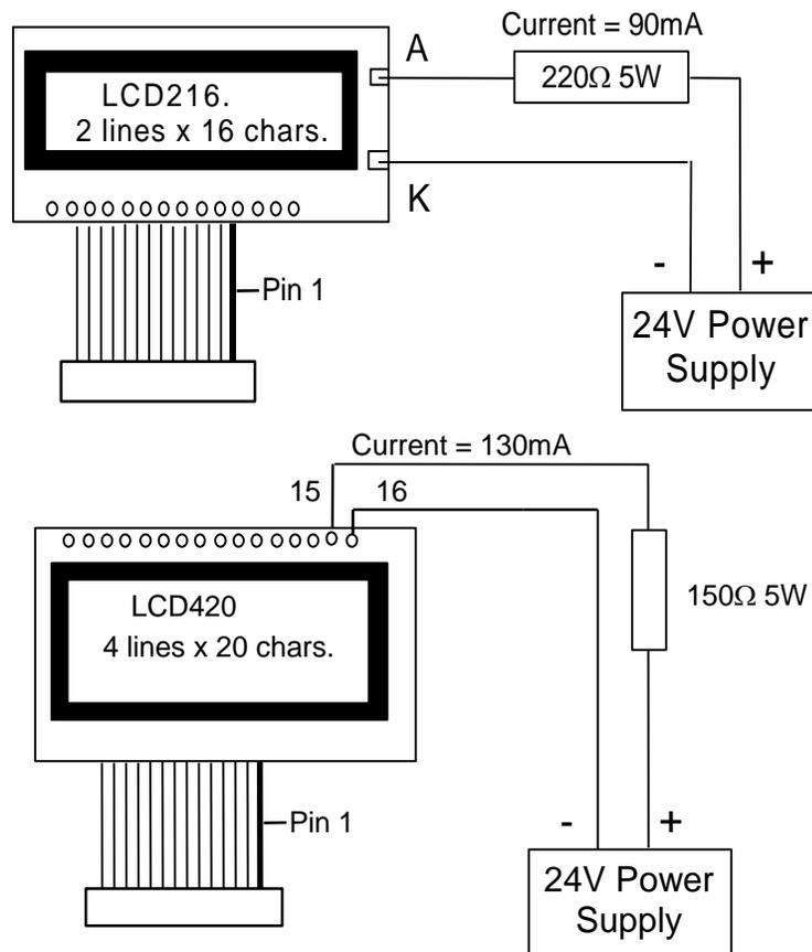
Figure 1.8 – Wiring of LCD216 and LCD420 backlight.
