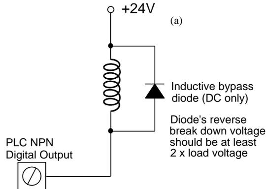
Figure 1.7 – Protective Solid State Output Against Inductive Kick.
