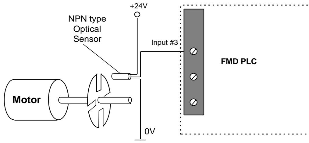
Figure 8.1 Setting Up a Simple Tachometer or Encoder
