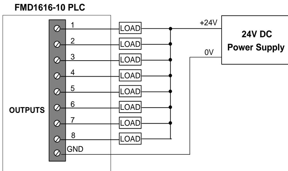
Figure 1.6 - Transistor Output Interfacing to Load
