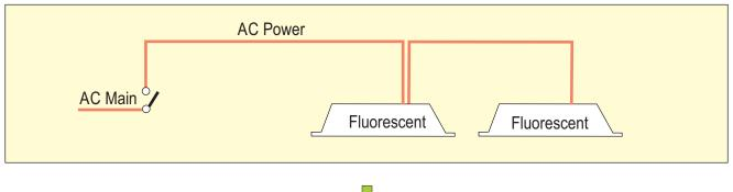
1) Replace flourescent fixtures with LED panels. Reuse the old L, N and Ground wiring.
