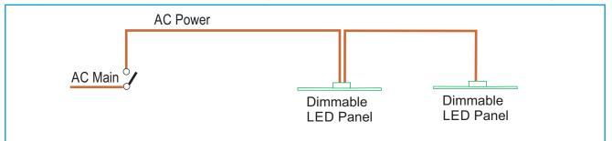
2) Cut the AC power supply line and connect to Alec's power Input and output. Connect 0-10V Dimming signal wires from Alec to the new LED panels Bypass the original manual switch to supply constant power to Alec.
